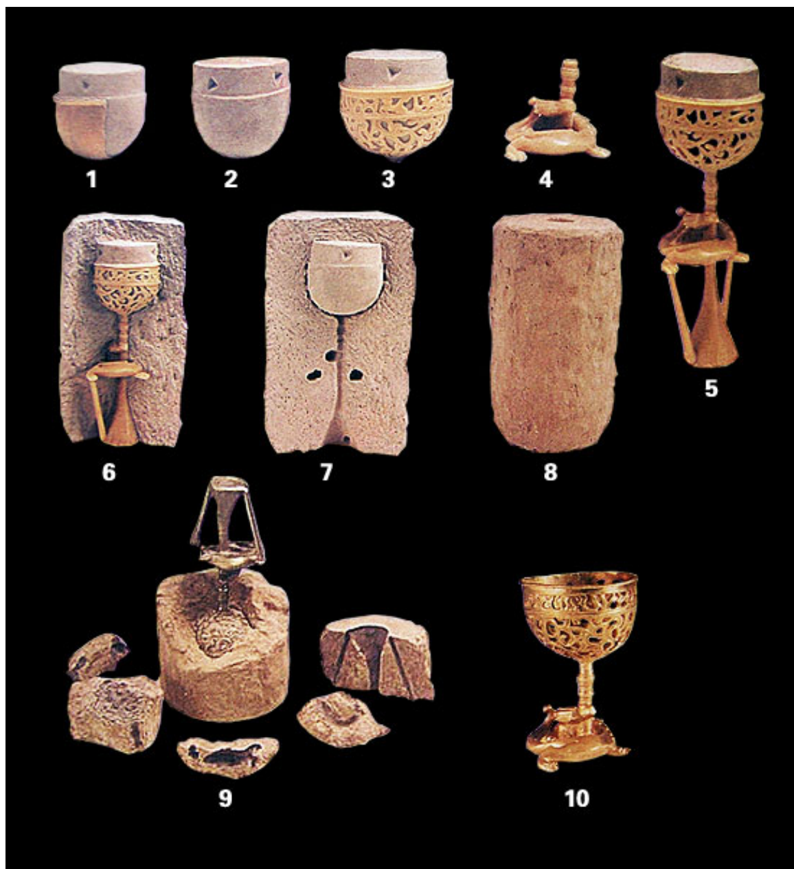
Figure 37: The complete lost-wax casting process for a bronze incense burner
